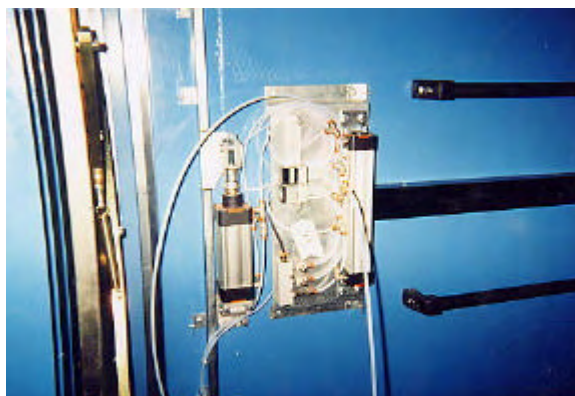
Pneumatic latches easily accessible for maintenance and repair
