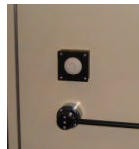
Internal air operated switch for solenoid lock release, designed to ensure no RF leakage or need for RF filters on the electrical wires
