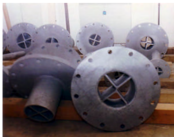
Large diameter pipe penetrations for generator exhaust gas in an EMPP (Electro-Magnetic Pulse Protection) bunker
