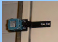
Electronic limit switch so door position can be monitored
