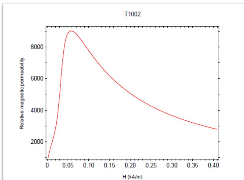
Figure 1: Permeability curve of a grade of Transil
