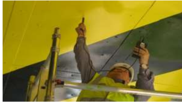
Vibration and fluctuating magnetic field survey for MRI scanner
